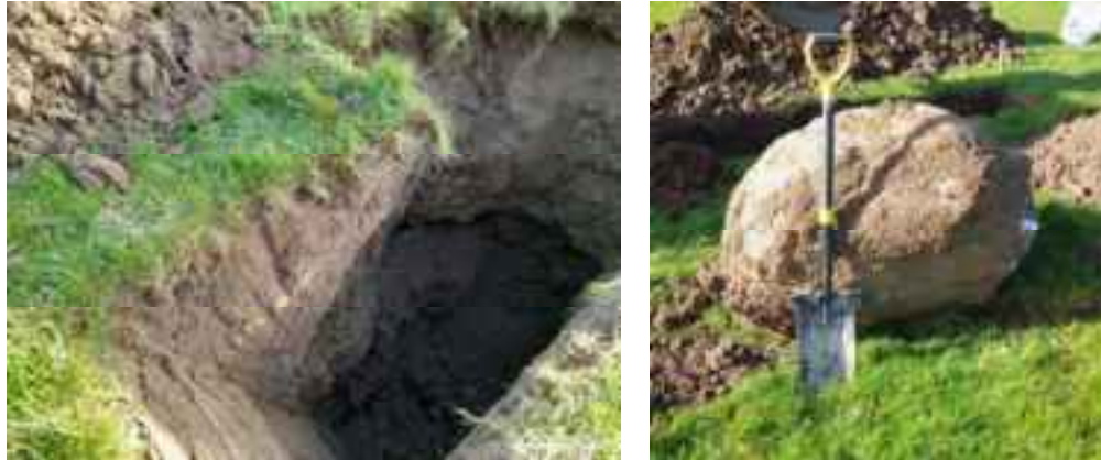
Figure 8A & 8B – Sidewall photo of TP05 showing SILT over dense GRAVEL at 2.0m (78.91m OD). Boulder found in pit at 1.80m measuring 1200mm.
