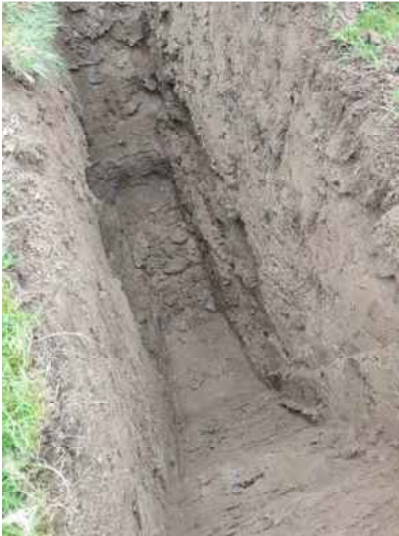
Figure 15 – Sidewall profile in BRE SA06. Pit walls unstable from 1.25m bgl.
